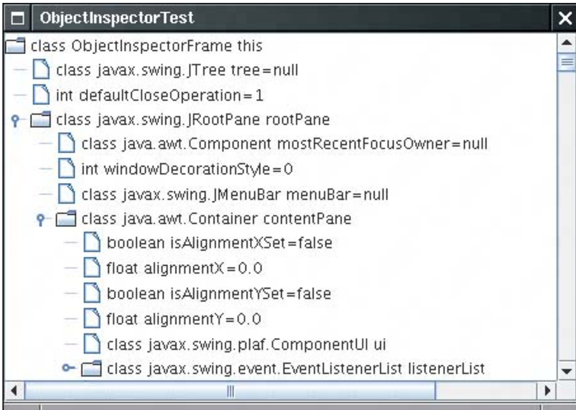
Figure 6-25. An object inspection tree
