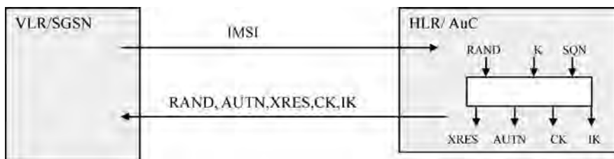
Figure 2-6. UMTS authentication. (Source: IP for 3G . Reproduced by permission of © 2002 John Wiley & Sons Ltd.)
