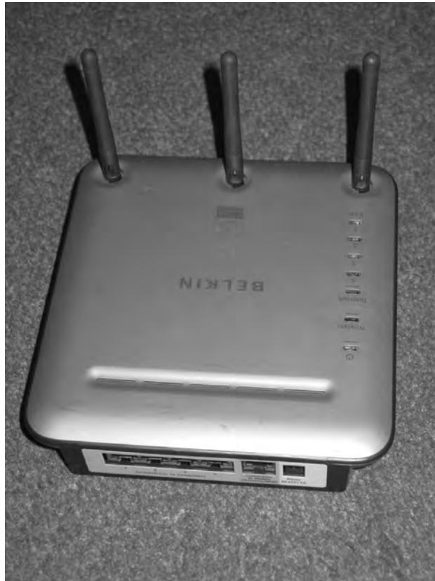
Figure 3-31. Pre-n router with triple diversity (author). (Source: Author. Reproduced by permission of © Dave Wisely, British Telecommunications plc.)
