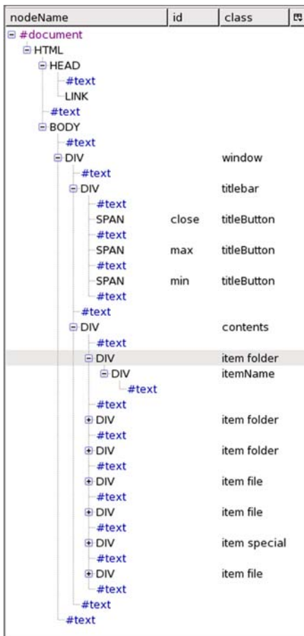
Figure 2.3 The DOM presents an HTML document as a tree structure, with each element representing a tag in the HTML markup.
