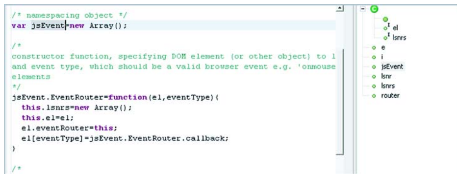
Figure A.2 The JavaScript editor plug-in for Eclipse provides rudimentary outlining support for JavaScript objects but doesn't handle the full object-based syntax.
