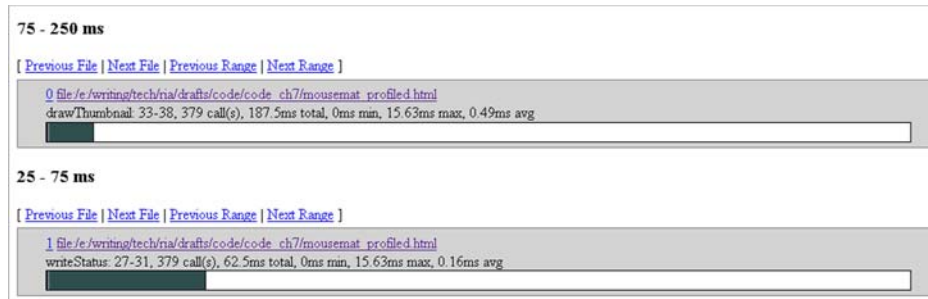
Figure 8.4 Fragment of the HTML profile report generated by Venkman showing the number of calls and total, minimum, maximum, and average time for each method that listens to the mouse movements over the mousemat DOM element in our example page.
